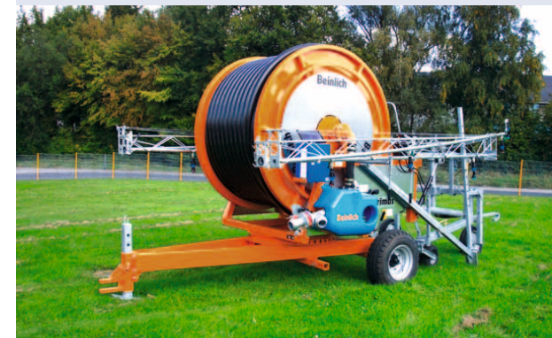
R 20 - 40 m zusammengeklappt an Primus 2000 sections folded on a Primus 2000, ready for lift up
