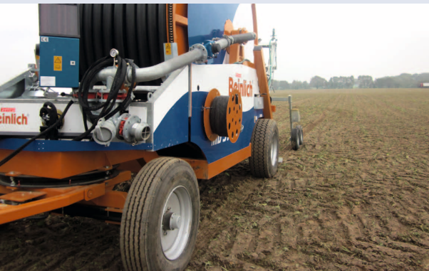
Räder vorne / tyres in front: 11R 22.5 16 Ply, hinten / in rear: 385/65 22.5 18 Ply
